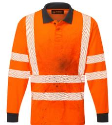
Pictured after Open Arc test showing incredibly intact fabric with ELIM result of 6,8cal/cm
